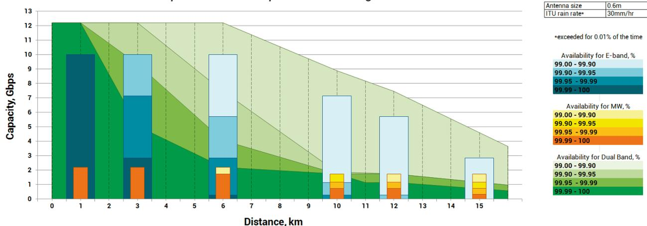
Chart 1 illustrates the systemic advantages of the dual band solution in terms of signal propagation. The four green areas on the chart show the resulting capacities of dual band solutions at various availability levels, depending on the link's distance.
